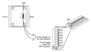
Figure 9. Models 2168A and 2168A/TB45 DIP switch orientation
